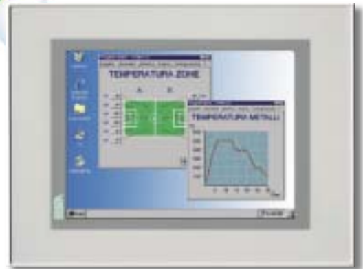
VT585CE LCD 65k Colores TFT 640 x 480 (10,4")
