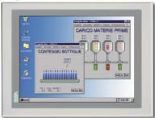
VT595CE LCD 65k Colores TFT 800 x 600 (12,1")
