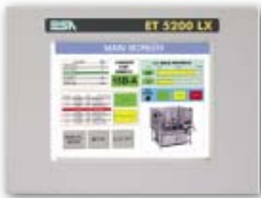
ET5200LX LCD 65k Colores TFT 640 x 480 (6,4")
